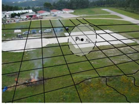
Fig. 4.24. Due to the uncertainties in sensor position and the cell resolution, one cell corresponds to a zone on the image plane (represented by the ellipse)
