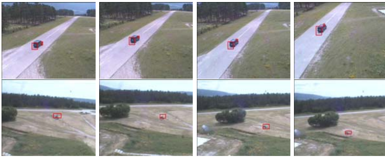
Fig. 4.15. The sequences show a moving car and other UAV of the fleet detected using a motion detection algorithm based on the image stabilization procedure
