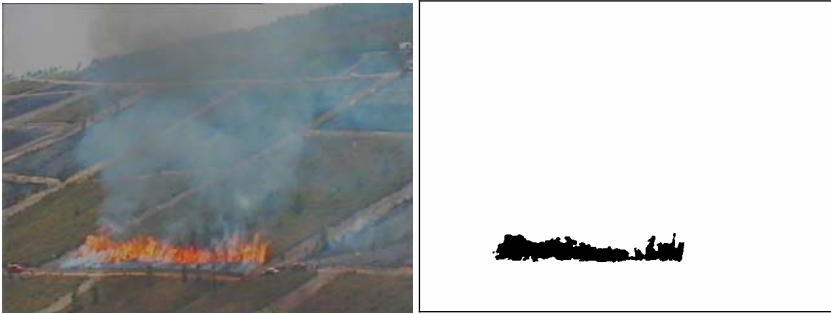
Fig. 8.6. Left: original colour visual image from a Gestosa fire experiment. Right: corresponding segmented image.
