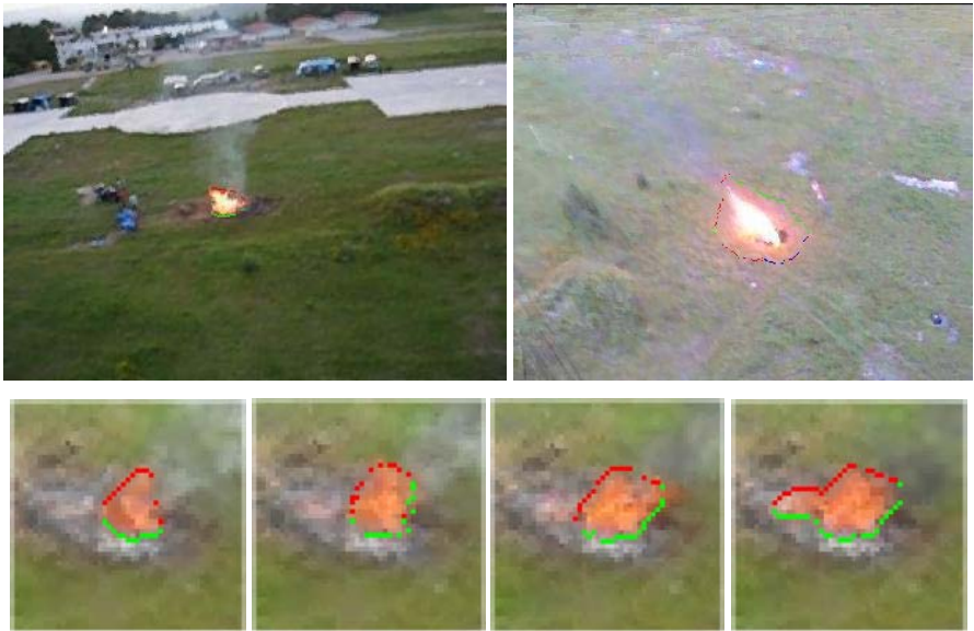
Fig. 8.22. Fire observation by using the MARVIN and Helivision-GRVC visual cameras. The fire front shape is marked on the images.
