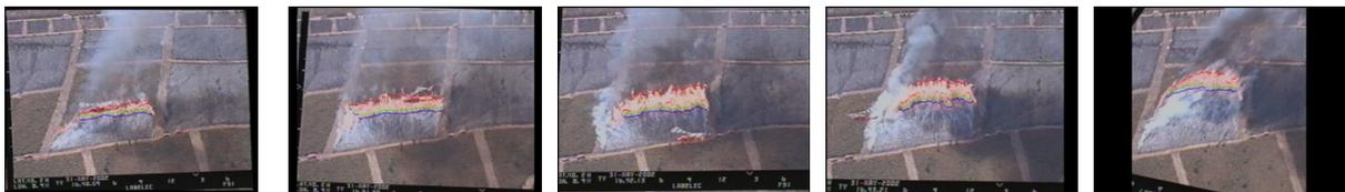
Figure 8: Frames 3, 44, 77, 144 and 219 of the aerial sequence gathered during the fire experiment 520, after automatic stabilization. The extracted fire front contour is also shown.
