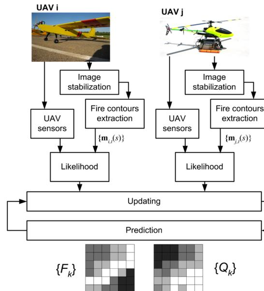
Figure 2: The system estimates two probability grids (fire presence and fuel at each cell). The state of the grids is estimated incorporating data obtained from the fleet of UAVs. The prediction step incorporates the increase in uncertainty due to the motion of the fire.
