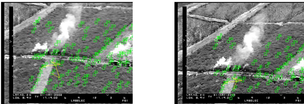
*Figure 5: Interest points extracted and tracked in two consecutive images to obtain a sparse image motion field. With this motion field, it is possible to compensate the image motion due to the vibrations.*
