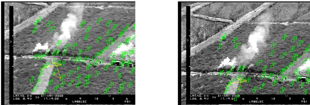
*Figure 5: Interest points extracted and tracked in two consecutive images to obtain a sparse image motion field. With this motion field, it is possible to compensate the image motion due to the vibrations.*
