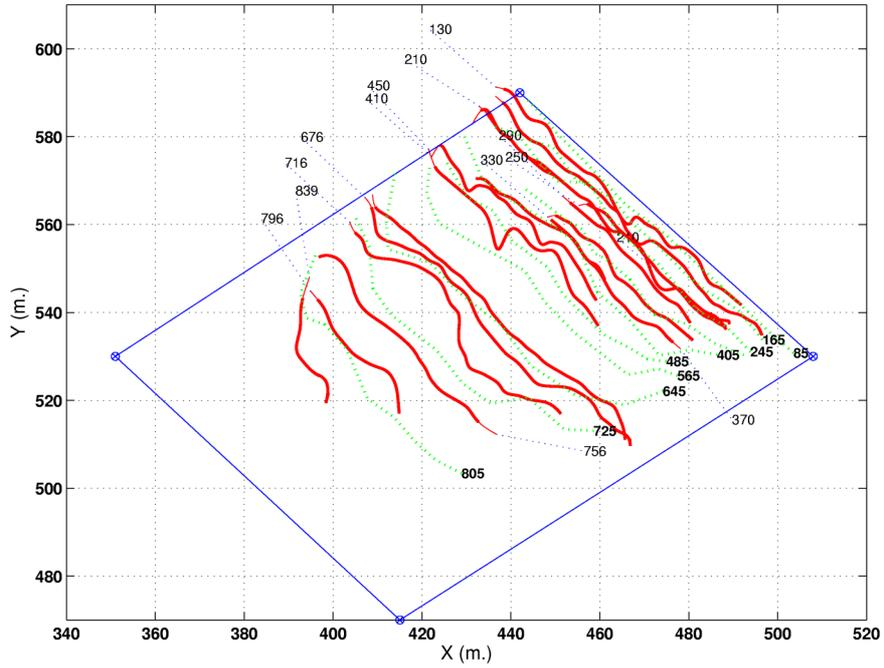
Figure 9: Evolution of the fire front (in georeferenced coordinates) for plot 520 estimated from the images gathered by the helicopter (solid) and compared with the front obtained with static cameras on ground (dashed).
