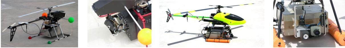
Figure 1: The UAVs carry mainly IMUs and GPS for navigation. Also, cameras on pan and tilt units for perception.
