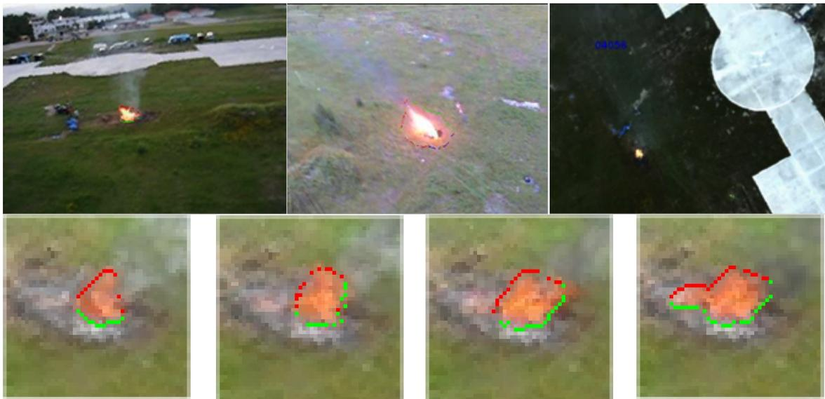
Figure 7: Top: left, image from Marvin, after stabilization and feature extraction; middle, image from Heliv after stabilization and feature extraction; right: image from Karma. Bottom: details of the extracted contours. Green: fire front. Red: top of the flames.
