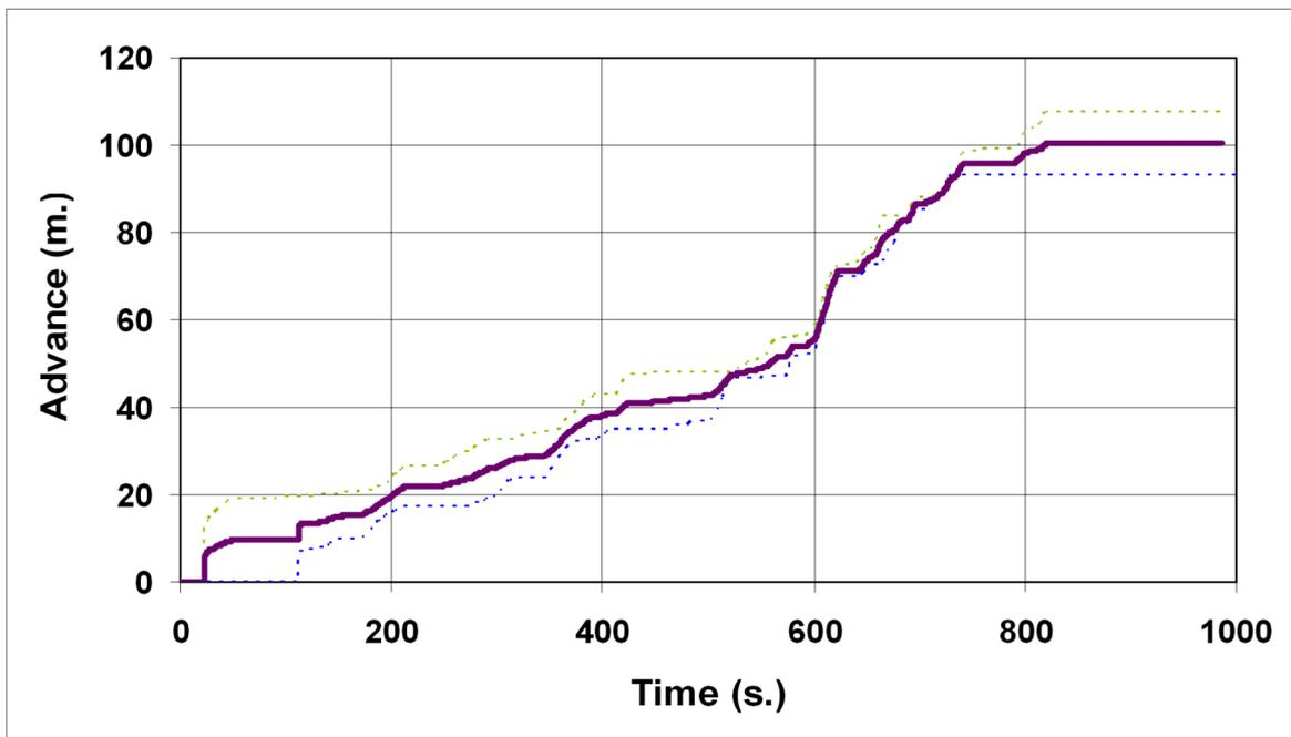
Figure 10: Evolution of the most advanced point of the fire front with respect to the coger firewall for experiment 520. Estimations from the aerial and frontal static cameras (dashed) and combined estimation (solid).
