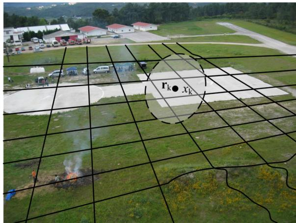
*Figure 3: The cells corresponding to a given pixel on the image can be obtained by a geolocation process. With this information, the probabilities of those cells corresponding to pixels segmented as fire will be increased.*
