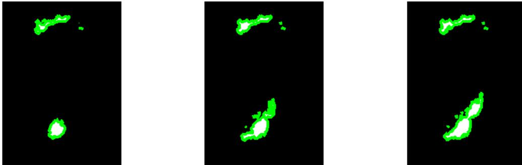
*Figure 4: The fire front shape can be obtained from the boundaries of the burnt zone. The figure shows the evolution of the burnt zone during one experiment.*
