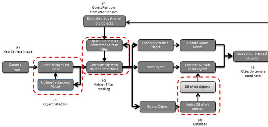
Fig. 4: System Overview of tracking objects using a single camera
