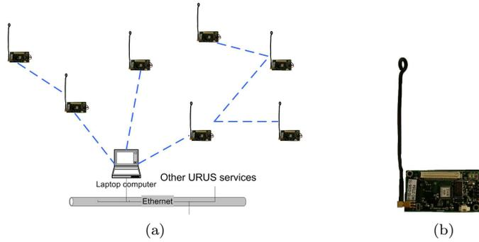
Fig. 9: Left: WSN architecture: the nodes can establish an ad-hoc network to relay information to a gateway. This information (messages indicating the power received from a mobile node) is processed in the gateway to obtain an estimation of the position of the mobile node. Right: WSN Mica2 node.
