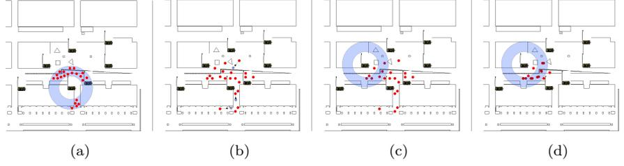
Fig. 10: Particles (red) are used to represent person hypotheses. (a) The filter is initiated when the first message is received by sampling uniformly from a spherical annulus around the receiver. (b) Particles are predicted at each iteration; map information is also taken into account. (c) New measurements are used to weight the particles. (d) Re-sampling maintains the number of particles bounded.
