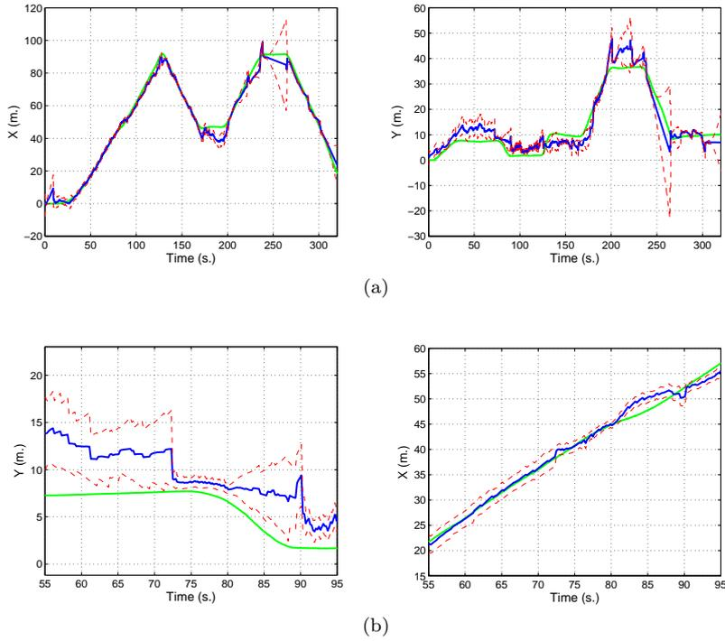
Fig. 21: Estimated position of the person (blue) compared to the position of the robot (green). Dashed lines represent the standard deviation of the estimation. (a) Complete trajectory. (b) A section of the trajectory. The person is following the robot with the same X coordinate up to time 80 seconds. Then the robot changes orientation. The person is separated from the robot around 3-4 meters.
