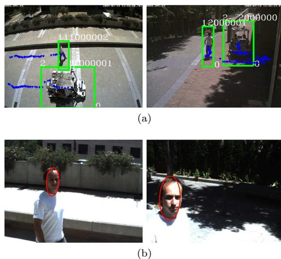
Fig. 20: (a) Tracks obtained by the camera network. (b) Tracks obtained by the camera on-board Romeo.
