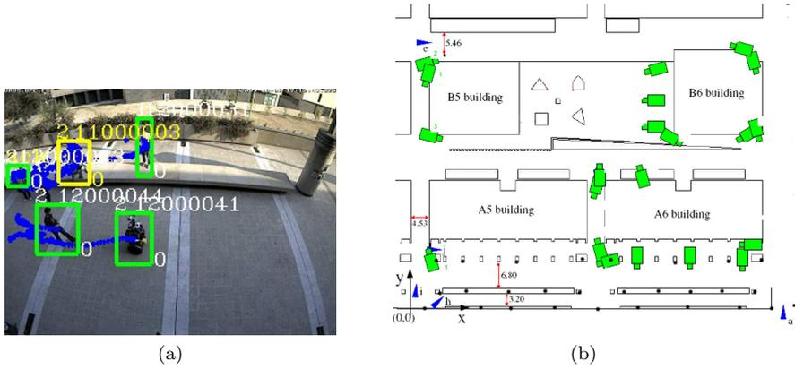
Fig. 14: (a) One of the robots (on the image marked as 12000041) guiding a person (12000044). (b) Scenario. The dimension is 100 by 100 meters, approximately. Cameras in green and Mica2 nodes as black dots.
