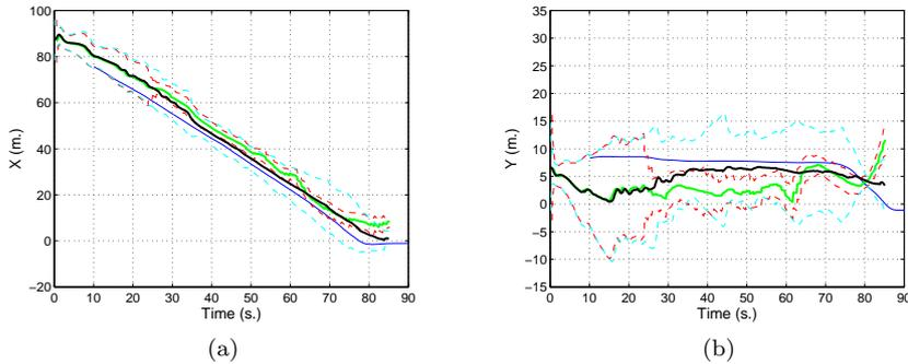
Fig. 19: Tracking using one on-board camera and the WSN. Black: robot alone. Green: robot and WSN. Dashed lines are the sigma intervals and the blue solid line represents the robot trajectory.
