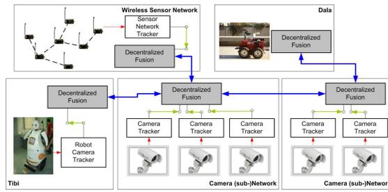
Fig. 3: A block description of the URUS perception system. The different subsystems are integrated in a decentralised manner through a set of decentralised data fusion nodes. Locally, each system can process and integrate its data in a central way (like the WSN) or in a distributed way (like the camera network). Some systems can obtain information from the rest of the network even in the case they do not have local sensors.
