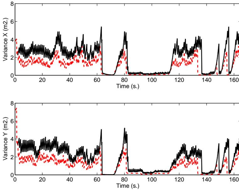
Fig. 22: Estimated variance by a central node receiving all the information (dashed and red) compared to the estimation in a decentralised node (solid and black).
