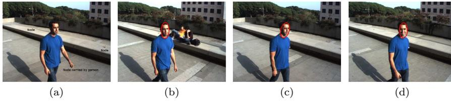
Fig. 18: (a) The person is carrying a Mica2 node during the experiment. (b,c,d) The robot is able to obtain local observations on the image plane of the face of the person.
