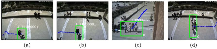
Fig. 16: Cross camera tracking (a) Person 11000001 on camera 11, (b) Person 11000001 correctly identified on camera 12 (c) Person 13000027 on camera 13 (d) Person 13000027 correctly identified on camera 12.
