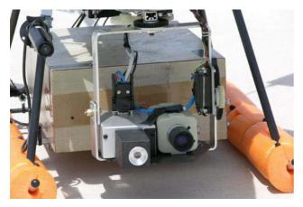
Fig. 6 Camera pan&tilt at COMETS helicopter.
