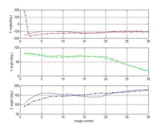
Fig. 8 Flight at Lousa airfield. X,Y,Z angles value evolution. Dashed: vision-based. Dotted: Pan&Tilt sensors. 3 images/second
