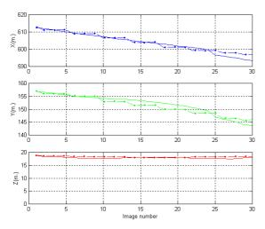
Fig. 7 Flight at Lousa airfield. X,Y,Z coodinates. Dashed: vision-based. Dotted: GPS. 3 images/second
