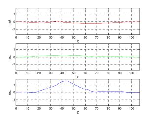
Fig. 3 Firewire camera trajectory in a 90° rotation over Z axis.
