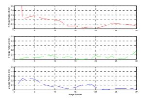
Fig. 9 Flight at Lousa airfield. X,Y,Z angles relative error. 3 images/second
