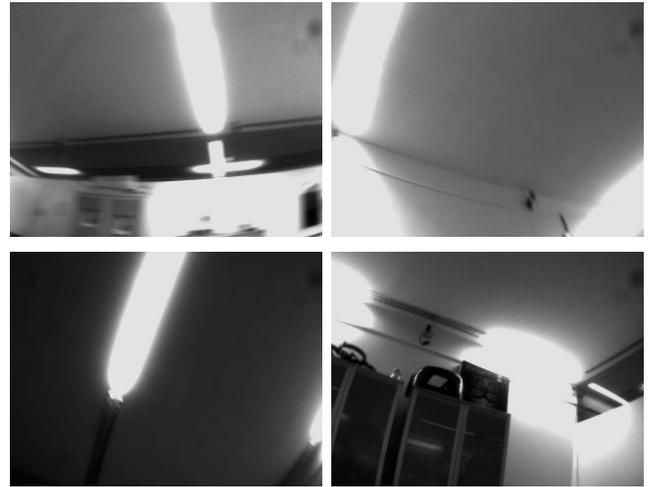
Fig. 6. Some examples of images gathered by the front camera during the experiment. It can be seen how images were taken at different illumination conditions. These images are downsampled to 10x8 before input the neural networks
