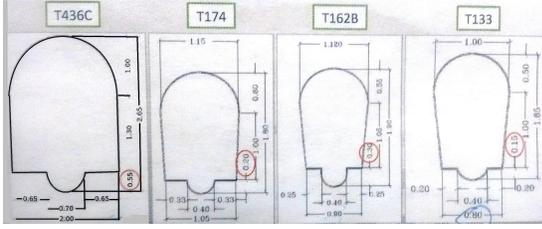
Figure 8: Sections of the sewers to be visited by the SIAR platform
