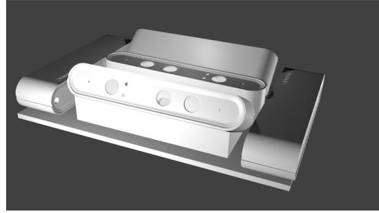
Figure 3: Proposed disposition of the cameras in the SIAR platform
