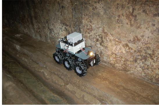
Figure 6: SIAR robot navigating in the sewers of the Passeig of Sant Joan
