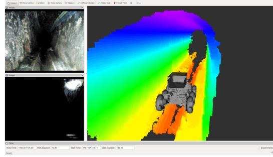
Figure 10: 3D local map reconstruction using RGBD data.
