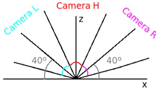
Figure 4: Detail of the angular disposition of central and lateral cameras for obtaining a continuous point cloud. Central camera (Camera H) is pointing towards the ceiling, while lateral cameras are rotated 40 degrees in the x axis
