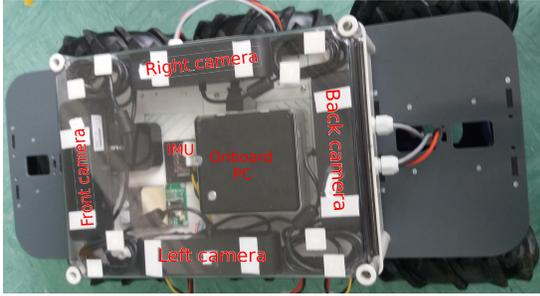
Figure 2: Detail of the sensors and computing unit in the SIAR platform
