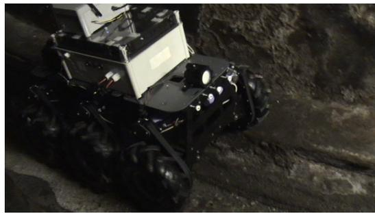
Figure 7: SIAR robot navigating in the sewers of Valencia street
