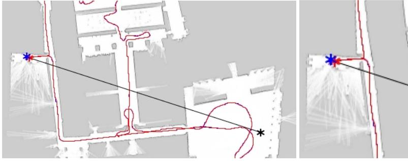
**Fig. 13** Black asterisk: Random initialization of MCL at Royal Alcázar of Seville. Blue asterisk: Ground truth initial pose. Red asterisk: Particle Injection first match: reinitialization of MCL hypothesis to this point. The subsequent estimated trajectory (red) is very close to the ground truth trajectory (blue).
