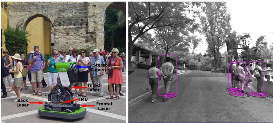
**Fig. 2** Left: the FROG robot platform. It shows the main platform and the positions of the sensors. Right: Estimation of persons poses on the screen, given by stereo cameras.
