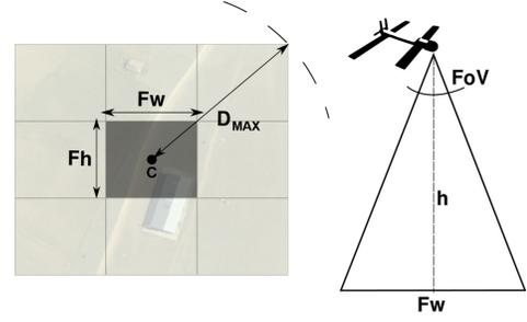
Fig. 2. Definition of the maximum distance ( $D_{max}$ ) used by MGRAPH for the neighborhood selection process. The footprint of the image ( $F_w$  and  $F_h$ ) can be calculated as a function of the Field-of-View of the camera and the flight height.
