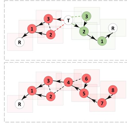
Fig. 3. (Top) A new image (called *trigger vertex*,  $T$ ) matches two graphs simultaneously. (Bottom) As a consequence, the secondary graph (top image, in green) is referenced to the primary graph (in red). After fusion, the secondary graph is deleted. Dashed lines represents *weak edges* meanwhile stroke lines represent *strong edges*.
