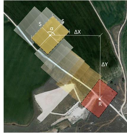
Fig. 4. Generation of the mosaic as an overlay in the GIS. A image  $i$  in a graph  $g$  is updated with the output generated by MGRAPH. A similarity transformation applies a translation  $(\Delta x, \Delta y)$ , a rotation  $(\alpha)$  and a scale factor  $(S)$  to the image  $i$  in relation to its reference frame  $(R)$  in the graph  $g$ .
