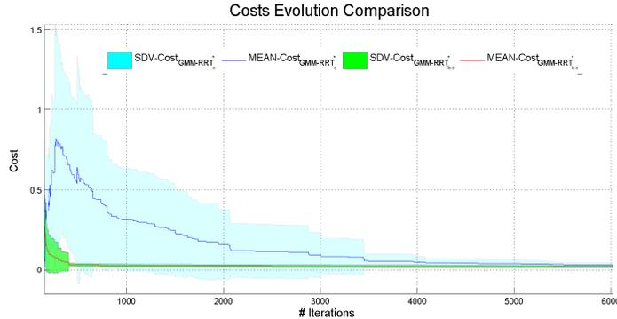
Fig. 1: Mean cost value and the standard deviation obtained for an GMM-RRT\* with (red and green, subindex  $bc$ ) and without (blue, subindex  $c$ ) GMM sampling bias.
