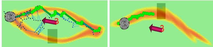
Fig. 5: “Avoiding a Person” task. Shaded area represents an obstacle. Left: Model includes 2 homotopies, used by GMM-RRT\*. Planning time: 3 secs. Right: Only right homotopy, used by GMM-RRT. Planning time: 100secs.
