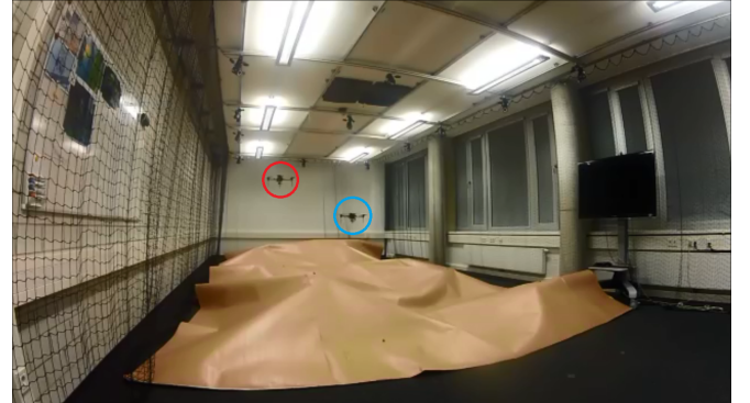
Fig. 1: Two quadcopters exploring an a priori unknown terrain profile with our proposed decentralized multi-agent exploration algorithm. They are equipped with an ultrasound sensor facing down to measure the distance to the floor.
