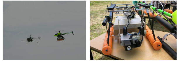
Fig. 1. Left, two UAVs of the COMETS fleet. Right: Electronic box and pan and tilt with the infrared and visual camera.
