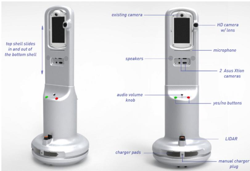
Figure 7.2: Final disposition of sensors on TERESA. The sensors used for navigation are the LIDARs (there is another one in the back, not shown here) and the XTion cameras.
