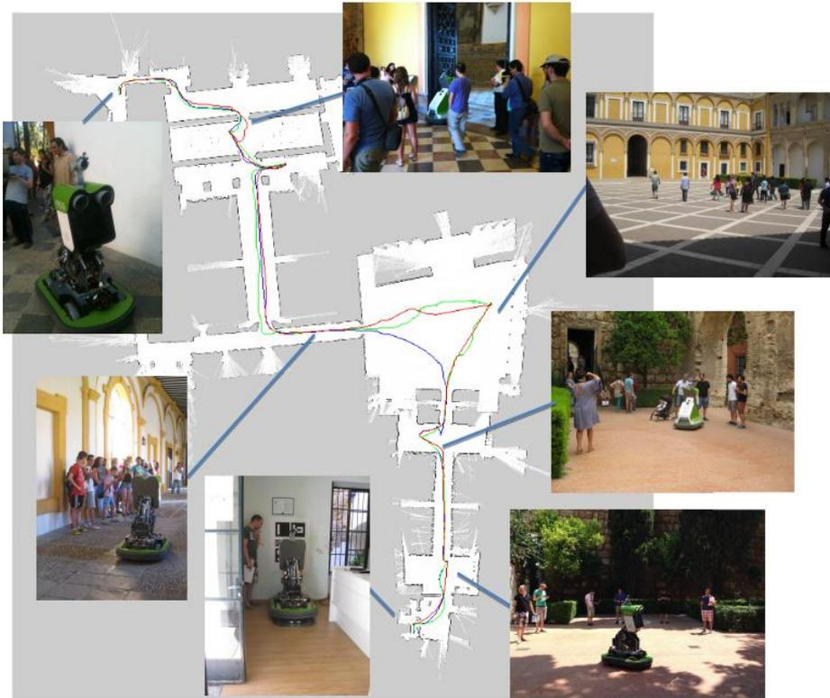
Figure 4.8: An overall view of the performed tours in the Royal Alcazar of Seville. Three different examples of the trajectories for the tour are shown in red, green and blue (the tour details depend on the time of the day, leading to some differences in the trajectories). Different photographs illustrate the different zones in the trajectory.
