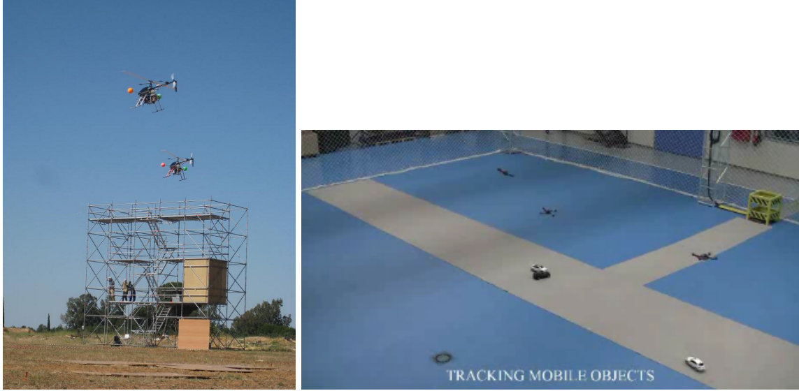
Figure 1: Multiple UAS can cooperate in tasks like surveillance and tracking. Left: two autonomous helicopters in a surveillance mission outdoors. Right: three quadrotors following targets in an indoor testbed. Robust mission execution requires to take into account uncertainties about the target’s position and motion model.
